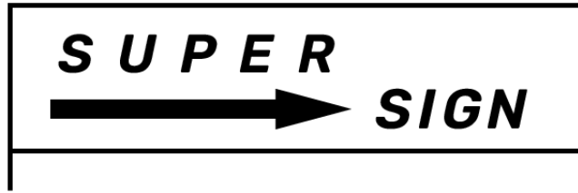
Figure 4: Sign area shall include vertical and horizontal spacing between letters conveying the sign's message.
